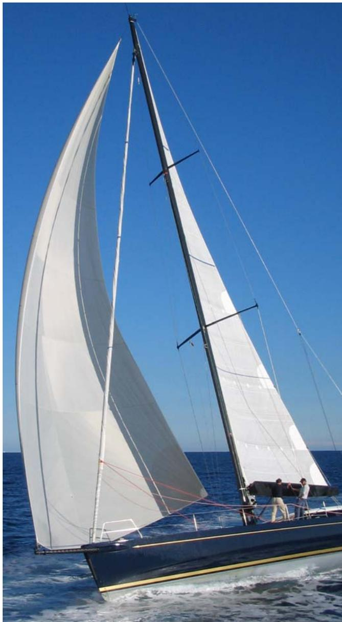
The Code Zero is a cross between a genoa and an asymmetrical spinnaker that is used for sailing close to the wind in light air. These sails are a must for distance races. Being nearly twice the size of a light No. 1 Genoa and made of much lighter weight material, a Code Zero will fill in the faintest of zephyrs. The greatest beneficiaries of these sails are modern boats that do not have overlapping headsails because Code Zeros have more than three times the sail area of a non-overlapping genoa.
