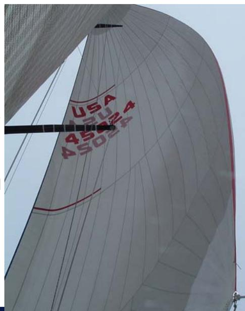
When the Code Zero is sheeted in tight, steer just as you would with a genoa — sail to the the tell tales. When the boat slows, fall off slightly until the boatspeed builds to about one knot above the wind speed. The highest these sails can be carried is 40 – 45 degrees apparent wind angle, but the boat will be a lot faster at slightly wider wind angles.
