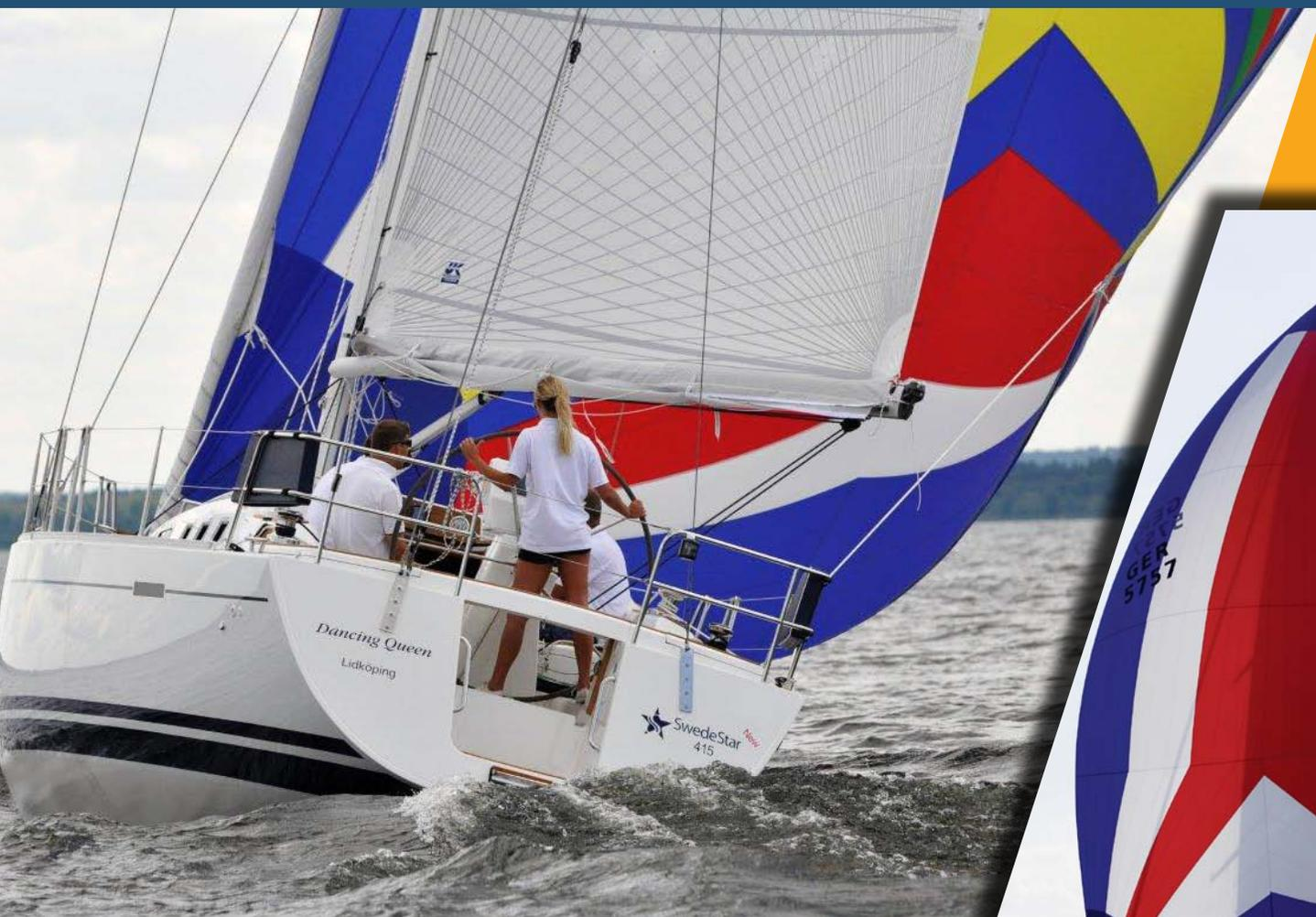
When the wind lightens, a UK Sailmakers Flasher is the ideal sail to keep you going downwind. It delivers almost as much pulling power as a full size spinnaker, yet it's so simple to use that it can be set, trimmed and lowered by one person.
