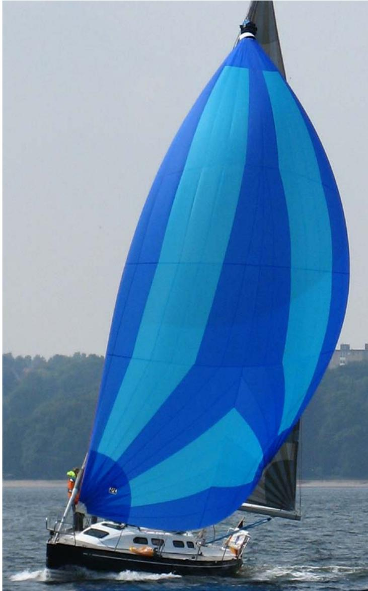
The Flasher's asymmetrical shape creates a stable and controllable profile; it's so stable you can even use it while using an auto pilot. In light airs, the sail can be carried as high as close reaching...in stronger winds you'll be more comfortable at broader wind angles.
